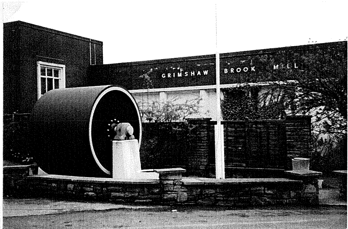
b. Paper Making Cylinder in Front of Grimshaw Brook Mill, Paper Envelope Plant
